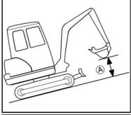
While going downhill, if the ground allows it, let the bucket slide on the ground.
