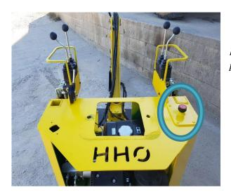
If need be, add oil by removing the 4 screws then the steel plate.
