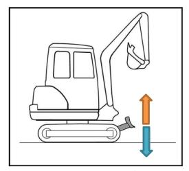
To lower the blade, push the front left lever (1) to the right
